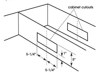
To vent through the roof with 3-1/4" x 10" rectangular vent, mark a line 1" and 5" from the back wall on the underside of the cabinet. Mark lines 5-1/4" to the right and left of the centerline on the underside of cabinet that connect the lines just drawn. Use a keyhole saw and saber saw to cut a rectangular opening for the ventwork. Repeat for the underside of the top of the cabinet.
